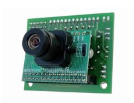
Figure 31. CMUCAM, low power alternative to web cam [From: Ref. 14].
